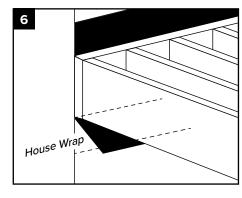
Install the house wrap and slide it up behind the remaining section of the sub-ledger tape. Then peel off the remaining release liner and smooth the tape over the house wrap.
