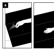
Once aligned properly, peel off the 10" release liner and smooth the tape down the wall.
