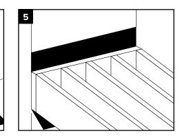
5. Install the ledger board and joist.
