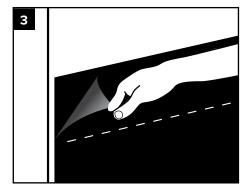
3. Peel off the 6" release liner and attach the tape across the width of the deck.
